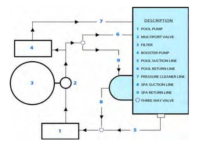
Note: This configuration would allow the spa to drain when pool pump is sucking from the spa and returning to the spa. Solve this problem by either:
