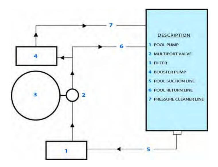
Tee the booster pump suction point after the filter and before any sanitizing devices, liquid chlorine feeders, acid injection points or salt water chlorinators.
